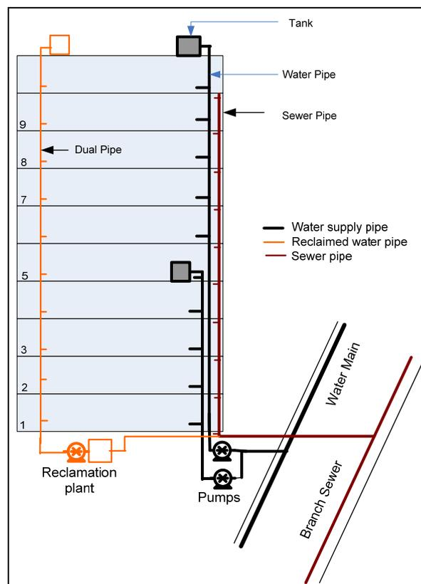
Figure 2: On-site wastewater system (Source: Sharma et al, 2005)
