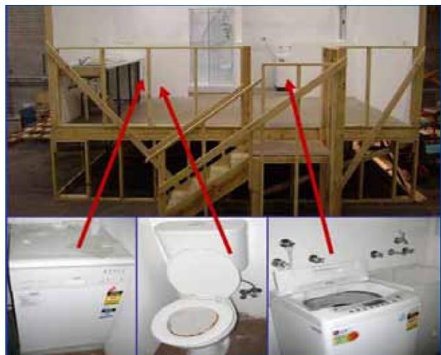
*This model house allowed researchers to control system variables and investigate the energy efficiency of different tank pumps.*
