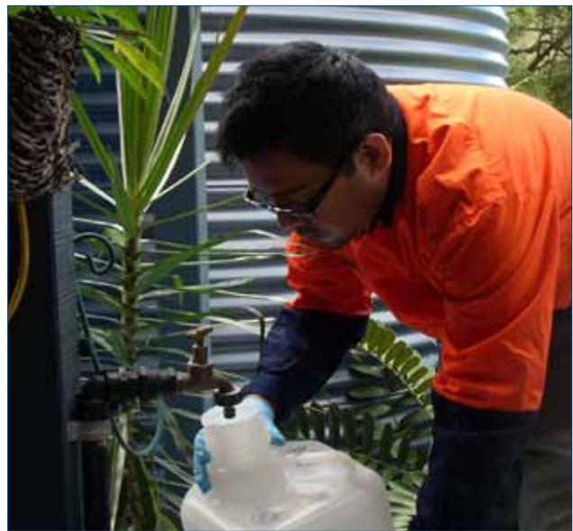
*An Alliance researcher samples rainwater tank water for testing.*
