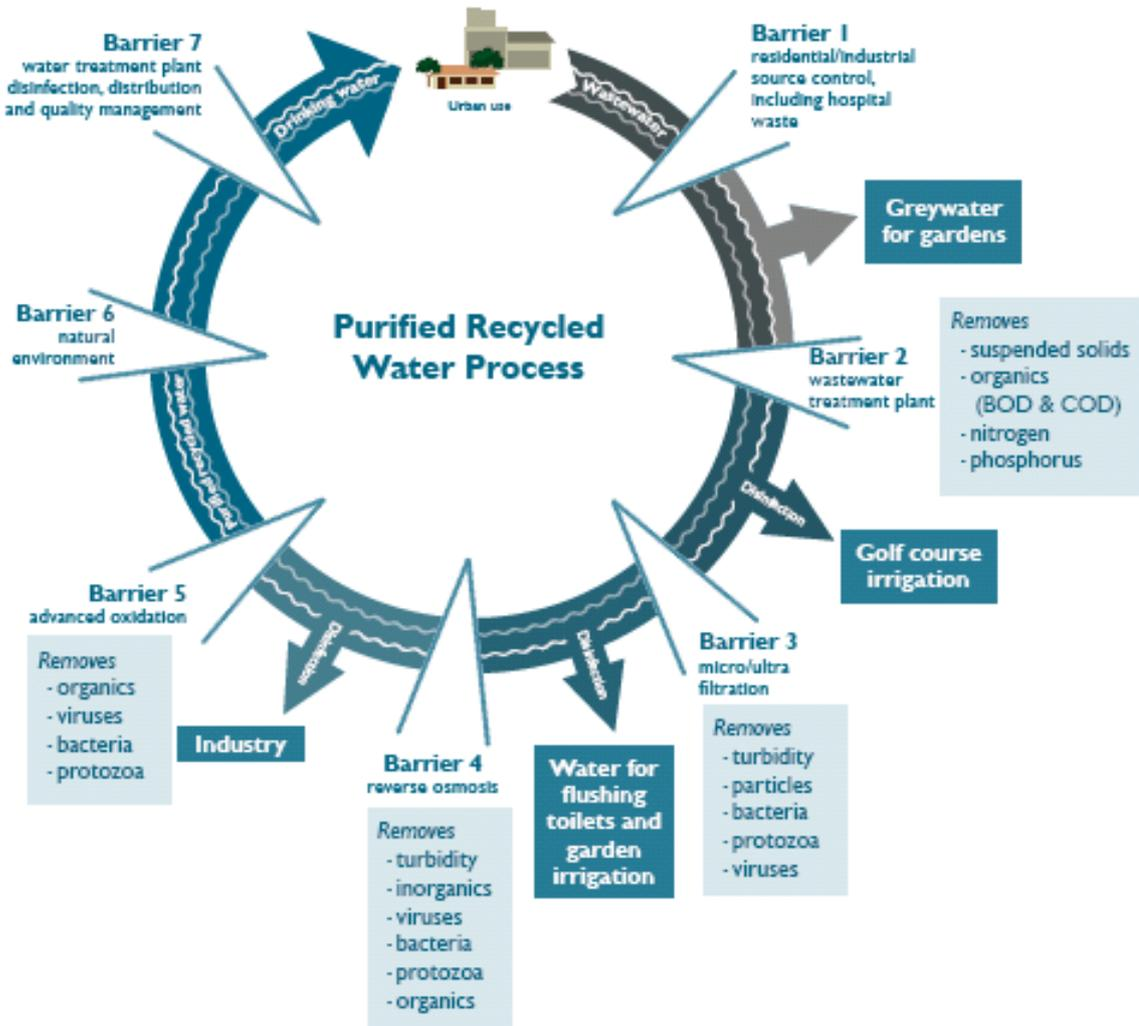
**Figure 1 Schematic of a Closed Water Loop Operation via the Seven-Barrier Treatment Process Employed in the Western Corridor Purified Recycled Water Scheme. (source; Queensland Water Commission Fact Sheet 4)**
